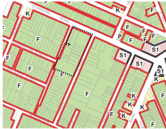
Figure 16: Extract from Marrickville LEP 2011 Floor Space Ratio Map (site outlined dashed) KEY: F = 0.6:1 P = 1.2:1 S1 = 1.5:1 K = 0.85:1
