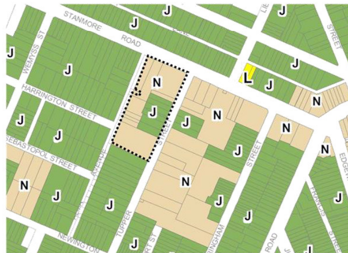
Figure 15: Extract from Marrickville LEP 2011 Height of Buildings Map (site outlined dashed) KEY: J = 9.5m N = 14m
